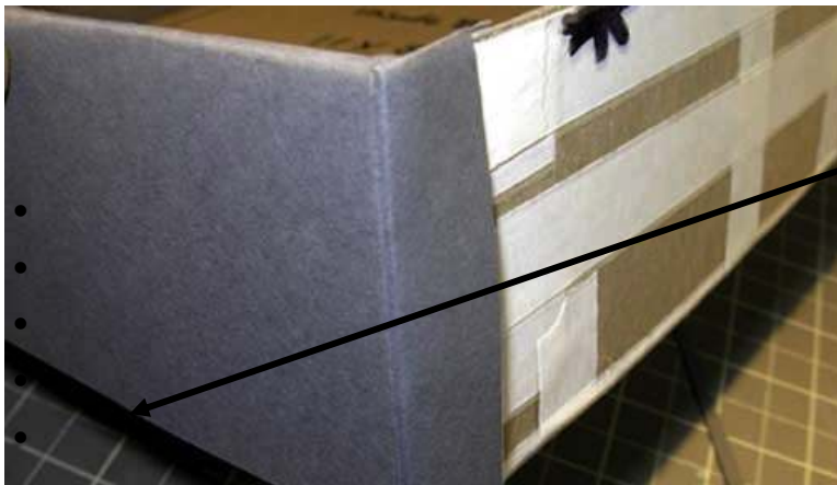
Outside edge of side covers do not fold under – they just reach to the bottom of the box side.
